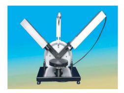
PhE-101D is a high speed discrete wavelength ellipsometer designed for measuring the refractive index and thickness of thin films. The PhE-101D takes quick and accurate readings due to its precision optical analyzer/detector and its stable mechanical design. The ellipsometer is supplied complete with integrated acquisition and analysis Windows software package, which further enhances the speed and ease of use of the instrument.
