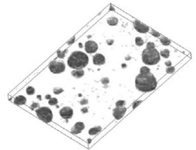
Silica nanoparticles within polymer matrix (nanocomposite material). Each individual image size is 20x40  $\mu\text{m}$ , spaces are 200 nm. Sample courtesy of Dr. Aliza Tzur, Technion, Israel.
