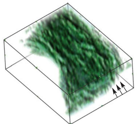
AFM tomography of resin embedded cyanobacteria. Photosynthetic membrane lamellae are clearly seen both on enlarged AFM image and on a 3D model (4.9x4.6x0.9  $\mu\text{m}$ , spaces between sections 50 nm). Sample courtesy of Dr. N.Matsko, ETH, Zurich, Switzerland.
